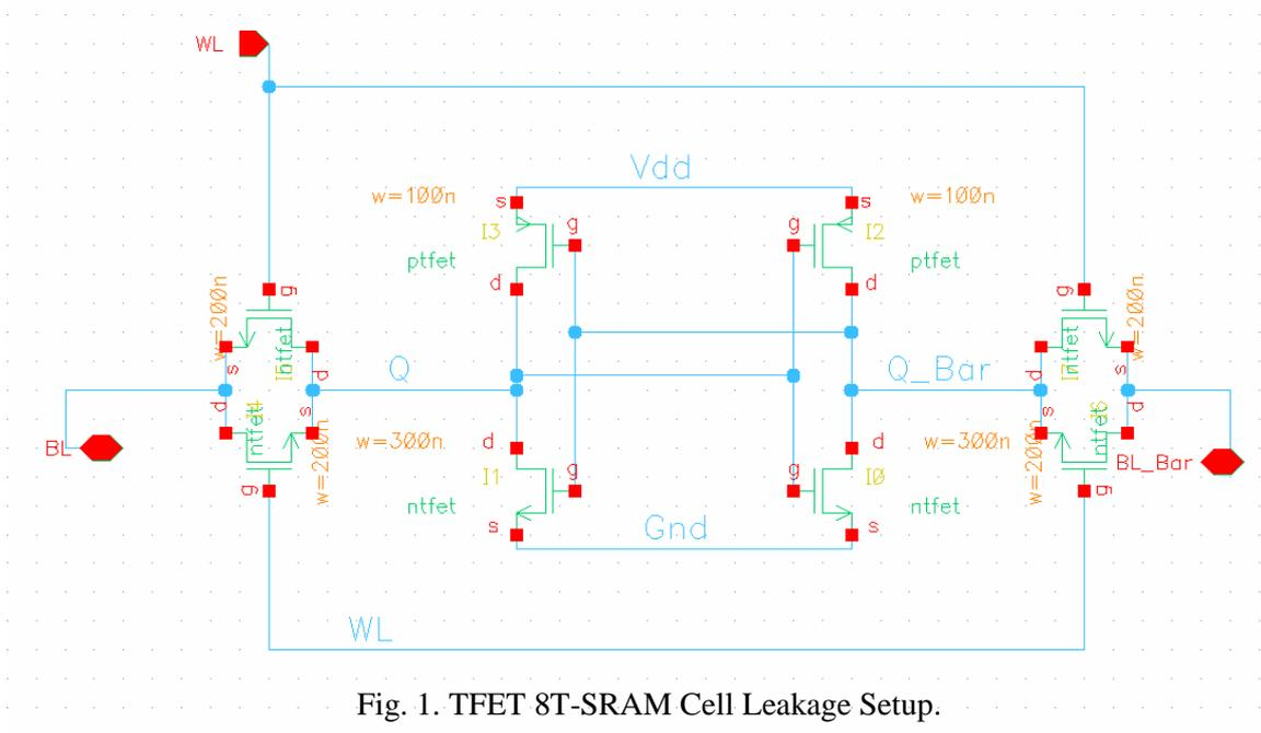
Fig. 1. TFET 8T-SRAM Cell Leakage Setup.
